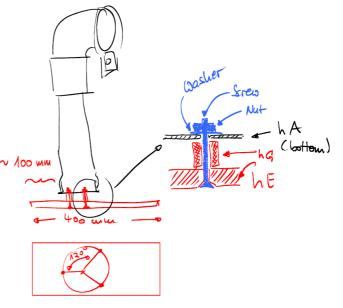
Now three holes have to drilled into the bottom end cap to match the holes in the base plate. Finally the parts can be assembled according to the drawing above.
